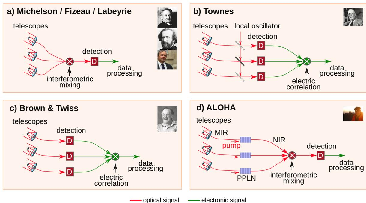
FIGURE 1 : Comparative presentation of the three classic configurations and the ALOHA concept (bottom right). Top left : the most common method uses the field correlation. The two intensity correlation measurements (direct and heterodyne) are shown top right and bottom left).
